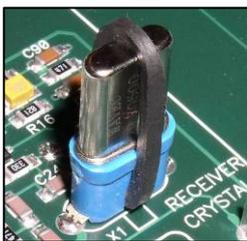
The RX-D is tuned to a single frequency by a crystal. The crystal can be custom made to allow reception of any frequency between 25.5 and 35.5 MHz. The receiver is pre-tuned at the factory but can be retuned later by Datawell to allow reception of other frequencies.
